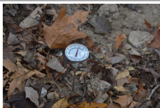
Soil thermometer at 5 cm depth.
