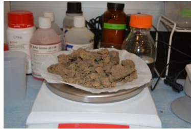
Weighing and drying a soil sample.
