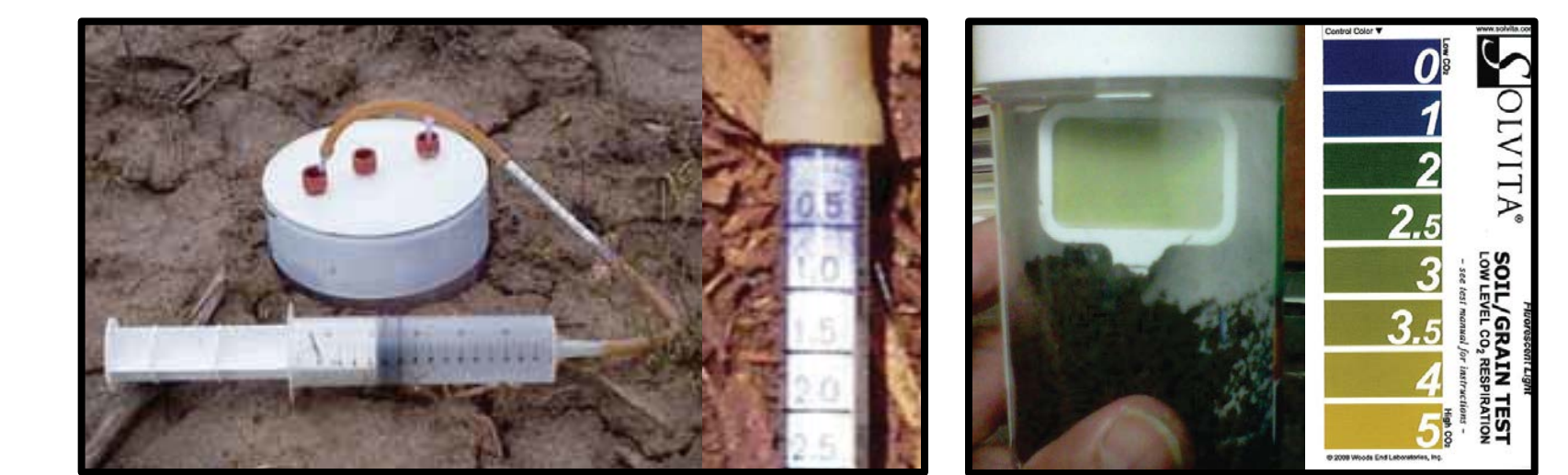
Figure 4. Measuring soil respiration in the field (Draeger tubes) and the lab (Solvita probes).
