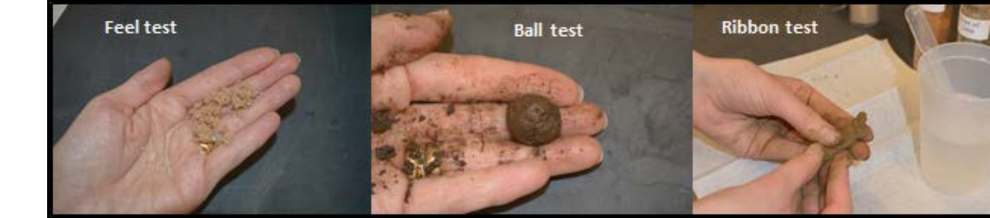
A. Qualitative methods to determine soil texture. The ability to make a ball or ribbon indicates higher content of clay.
